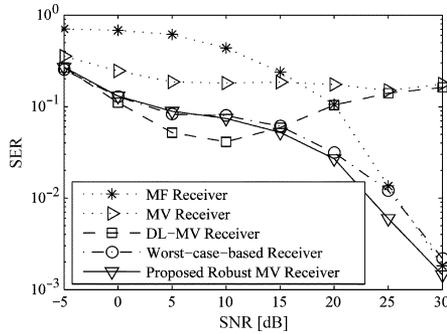
Fig. 2. SER for varying SNR ( $J = 40$ ,  $\sigma_e^2 = 0.2$ ,  $\text{INR} = 20$  dB).
