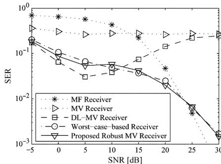
Fig. 3. SER for varying SNR ( $J = 60$ ,  $\sigma_e^2 = 0.2$ ,  $\text{INR} = 20$  dB).
