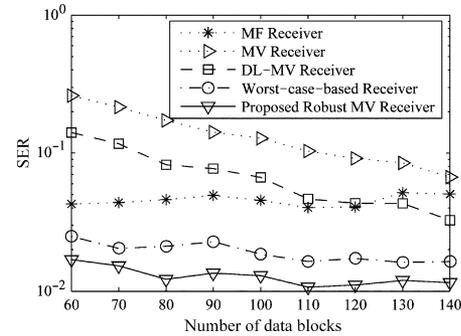
Fig. 4. SER for varying  $J$  ( $\sigma_e^2 = 0.2$ ,  $\text{SNR} = \text{INR} = 20$  dB).
