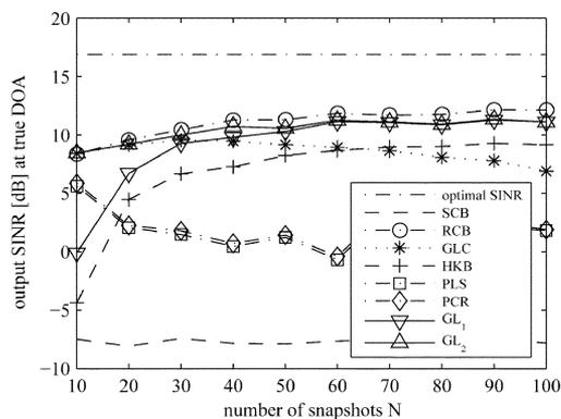
Fig. 2. Mean output SINRs for varying  $N$ .
